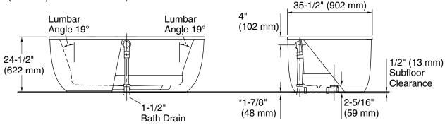
\*Allow for appropriate clearance in subfloor for drain tee clearance. Note: Horizontal PVC pipe and tee shown, not included.
